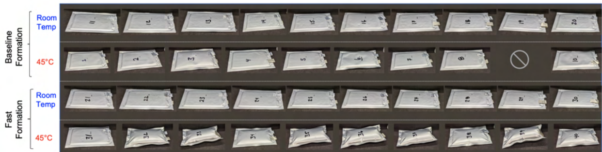
Figure B.26: Images of pouch cells taken after aging. Cell #9 has been excluded from the study due to tab weld issues.
