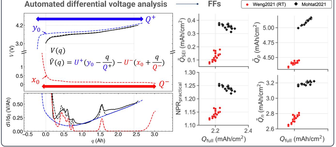
2. Physics-based formation models set a foundation for interpreting FFs, developing new FFs, and enabling model-based control of formation protocols.<sup>2</sup>
